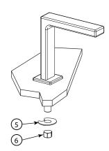
Insert spout base nipple into center hole in lavatory or counter top. Install stainless washer (5) nut (6) on spout nipple and tighten
