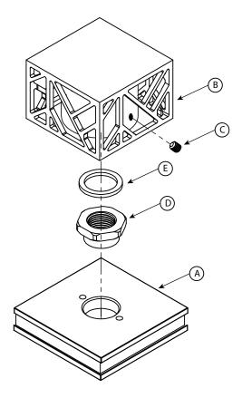
Place the pre-assembled base (A) over flush mount. Align base and secure using centering nut (D). Connect the pre-assembled cage handle (B) on to broach then tighten set screw (C) for final assembly.
