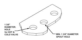
Should a counter top need to be drilled, please reference the diagram above.
